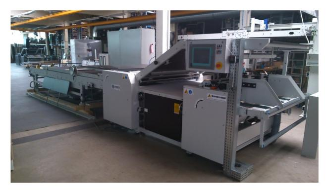
semi-automatic laminating machine, designed for semi-automatic laminating offset printed sheets, with a wide range of different carrier sheet. Used to produce high-quality, sales-promoting displays and packaging.
