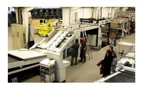
The glue rollers are easily cleaned within 5 minutes. Therefore only water is needed. In addition, it is equipped with the on-the-Fly' mode, that is, that there is no mechanical alignment of the sheet leading edge is required. Over the print sheet is aligned by a special page mark. The printed sheets are detected optically and electronically adjusted.
